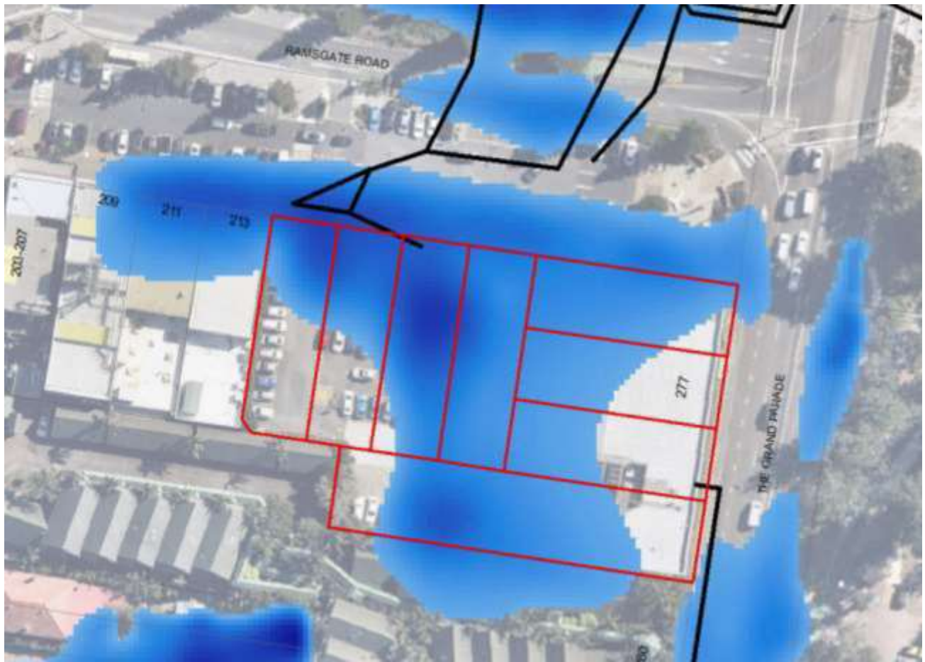
Figure 1: 1% AEP Flood Extent Map (dark blue indicates greater depth of water and pale blue indicates shallower depth, thick black line indicates approximate location of the existing drainage network)
